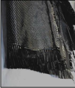
**Fig 2.1** Carbon Fiber Fig
