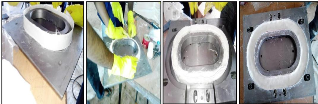
**Fig 5:** Folding Of Ply **fig 6:** Placing the First Ply **fig 7:** Assembling Die **fig 8:** Final View Before Curing
