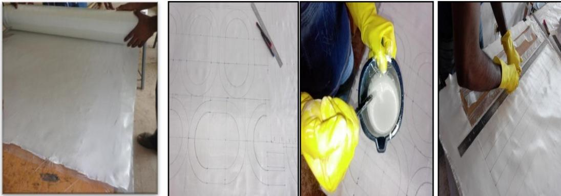
**Fig 1:** Glass fiber, **fig 2:** Marking window as per dim, **fig 3:** Matrix Mixing, **fig 4:** Cutting the Plies
