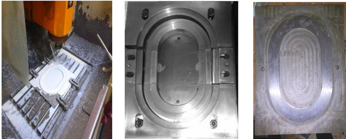
Fig 3.1 CNC Milling of Punch plate, Fig 3.3 Final Assemble of mold, Fig 3.4 punch plate
